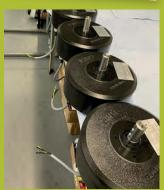
The magnet rotor is made up and fitted into the casing followed by seating and sealing the lid. The generator is then tested to ensure is has the correct output including a high voltage insulation test to prove long-term durability.
