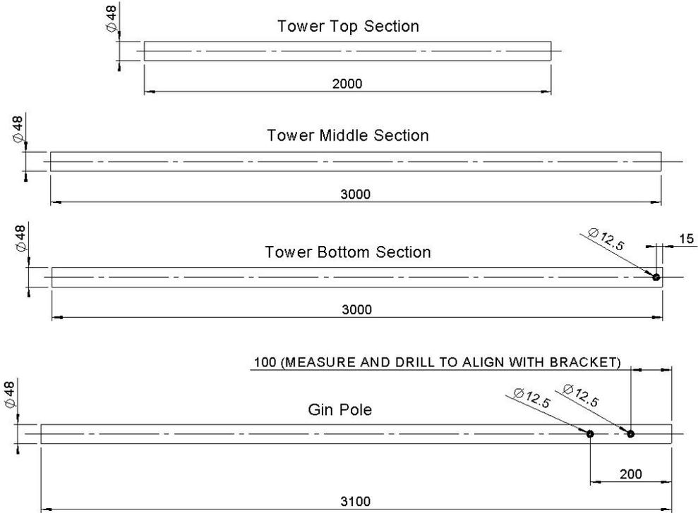
**i** Drill the poles as shown above except for the outer hole of the gin-pole. This should be marked through from the ground anchor point fixing during the first trial tower raising to ensure accuracy and ease of later fitting.
