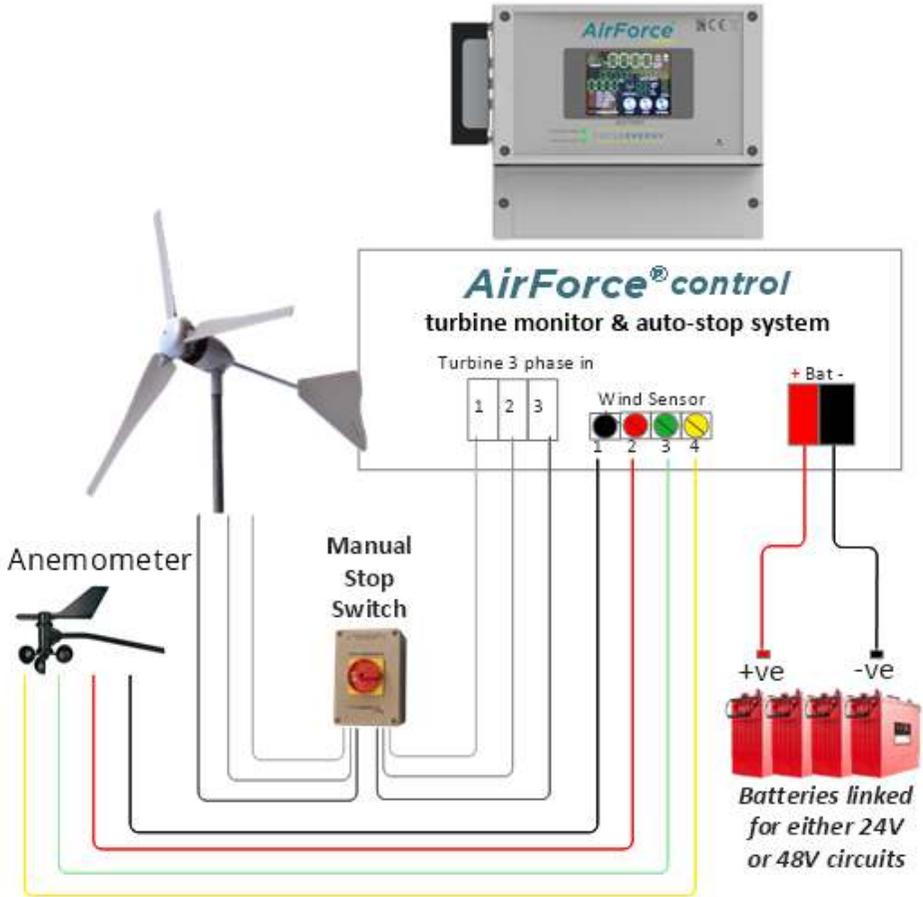
Figure 2 - Generic 24V or 48V circuit diagram
