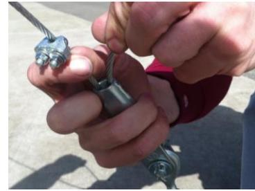
Connect the wedge socket onto the eye-end of the turnbuckle using the locating pin and securing split-pin.
