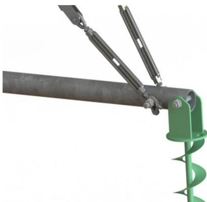
**i** Extend the turnbuckles to their maximum length prior to connecting to the guy-ropes to provide maximum adjustment when it comes to tightening the turnbuckle.
